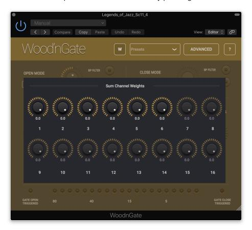
The Channel Weights Panel is shown when pressing the "W" button. This button is only visible when the plugin is inserted on a track with more than 2 channels.
