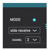
The audio from the side chain track (Base drum ...) will now be sent to the receiving Wood'nGate (Bass guitar) and be used as gate analysis signal which determines the open/close state on that track's audio.
